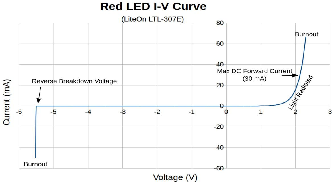
In a great simplification, a diode is a one-way valve for electricity; it lets current flow in one direction (forward direction) and not in the opposite direction (reverse direction). In reality, it is more complicated. A voltage applied in the forward direction must exceed a threshold value before the current flows. Beyond that value the current increases very rapidly for small increases in forward voltage. For LEDs that threshold voltage depends on LED color, but is usually around 2 V.
