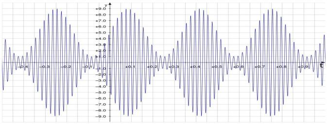
A device (**demodulator**) that extracts the lower frequency tone from this wave is easily constructed. This process can therefore carry information about the tone. If instead of this constant tone, the varying tones of music or voice were used for the modulation, we would have a method to send music or voice information over the carrier wave. This is how AM (**amplitude modulation**) radio works.
