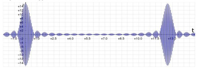
The pulses are now twice as far apart. Thus, we see that the more closely spaced the component frequencies, the farther apart the pulses become vs. time. An infinitesimally close spacing of frequencies corresponds to an isolated pulse.
