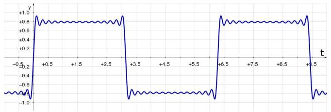
With an infinite number of terms, this would become a perfect square wave except for an infinitesmally narrow 9% overshoot at each jump. (Functions without discontinuous jumps are represented without such overshoots.)
