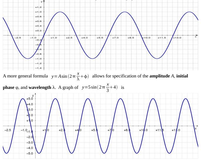
This time the sine curve peaks at  $\pm 5$  *y*-units, repeats every 3 *x*-units, and has a value  $y=5\sin(4)=-3.78$  at x=0, 3, 6, ...
