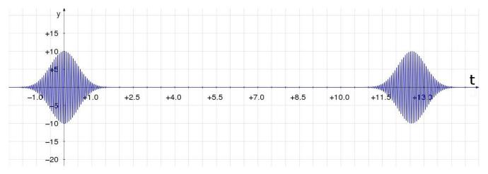
The pulse width has doubled. **In general, the pulse width varies inversely with envelope function width. A narrow pulse width corresponds to broader spectrum of frequencies.**
