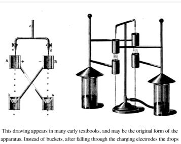
apparatus. Instead of buckets, after falling through the charging electrodes the drops fall into metal funnels which collect the charge but let the water through. This machine is equipped with Leyden jar capacitors (*cylindrical objects at base*) which store the charge
