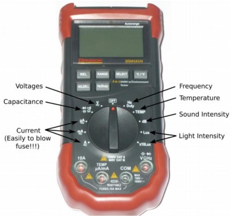
resistance mode rather than one of the other possible modes. Resistance is a measure of how much a circuit opposes the flow of electricity. The meter puts a gentle known voltage across the circuit and measures the current flow. It then uses Ohm's Law to report a resistance value.
