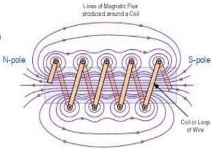
in the drawing have current flowing away from the viewer while the bottom of those turns have current flowing toward the viewer. We conclude:
